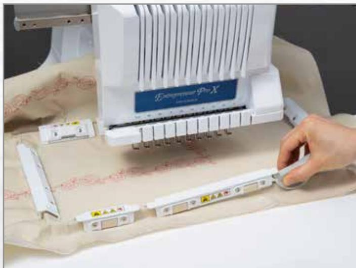
Included magnet lifter, easy to remove the magnetic pieces
