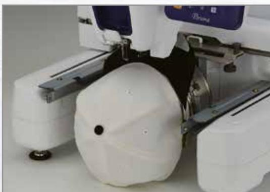
Set cap directly onto the machine
