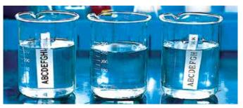
Water and chemical resistant: Glass plates with laminated labels attached were immersed in water and various chemicals for 2 hours. The text was unaffected.
