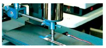
Abrasion resistant: After 1kg of sanding device was passed over the laminated labels for 50 times, the text was unaffected.
