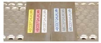
Temperature resistant: laminated labels were subjected to temperatures ranging from -80°C to +150°C for 240 hours and the text was unaffected.
